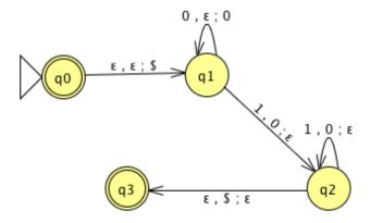
**Definition** A **pushdown automaton** (PDA) is specified by a 6-tuple  $(Q, \Sigma, \Gamma, \delta, q_0, F)$  where Q is the finite set of states,  $\Sigma$  is the input alphabet,  $\Gamma$  is the stack alphabet,
