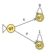
Prune this diagram to get an equivalent DFA with only the "macro-states" reachable from the start state.
